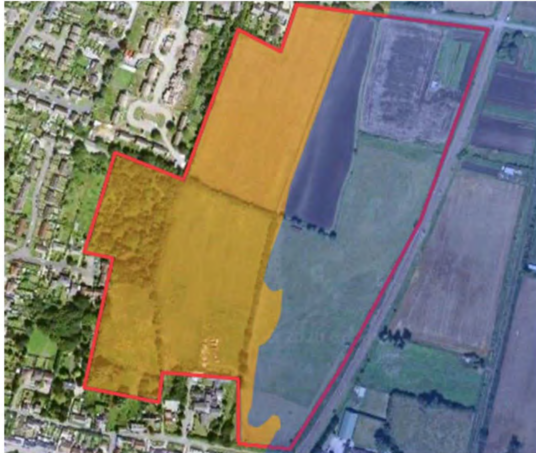
Fig.3.3 Potential developable Area beyond the modelled 1 in 100 year plus climate change maximum flood extent in defended scenario (WSP, 2019)
