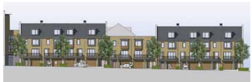
Fig 14: Illustrations of elevations showing what the overall street frontage will look like. It is important to recognise that the street will not be seen in this way when built, but this type of drawing will help demonstrate how the design of the elevations creates a cohesive character and sense of place. (John Thompson and Partners, 2009)
