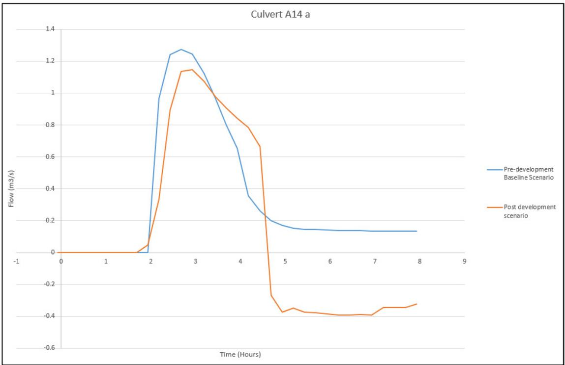
**Graph 1 – Flow through culvert A14\_a in both the Pre Development scenario and Post Development scenario**
