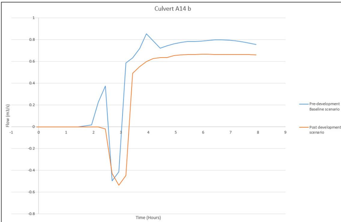
**Graph 3 – Flow through culvert A14\_b in both the Pre Development scenario and the DG2 and Post Development scenario**
