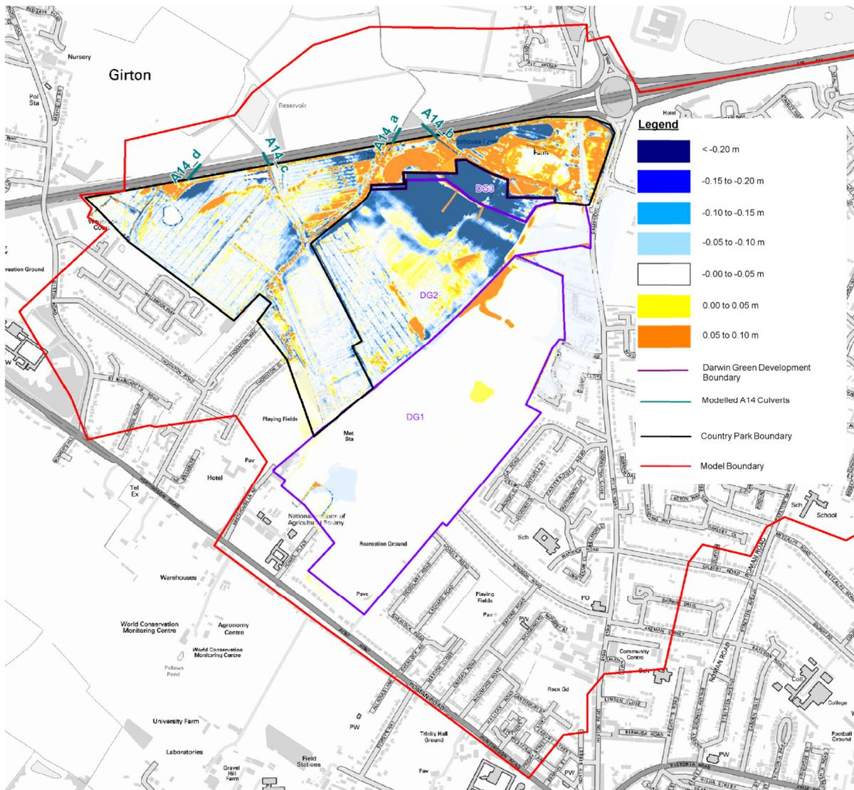
**Figure 4 – Depth differences in metres between the modelled Pre-development scenario and Post Development Scenario (for 1 in 100 year plus climate change event)**
