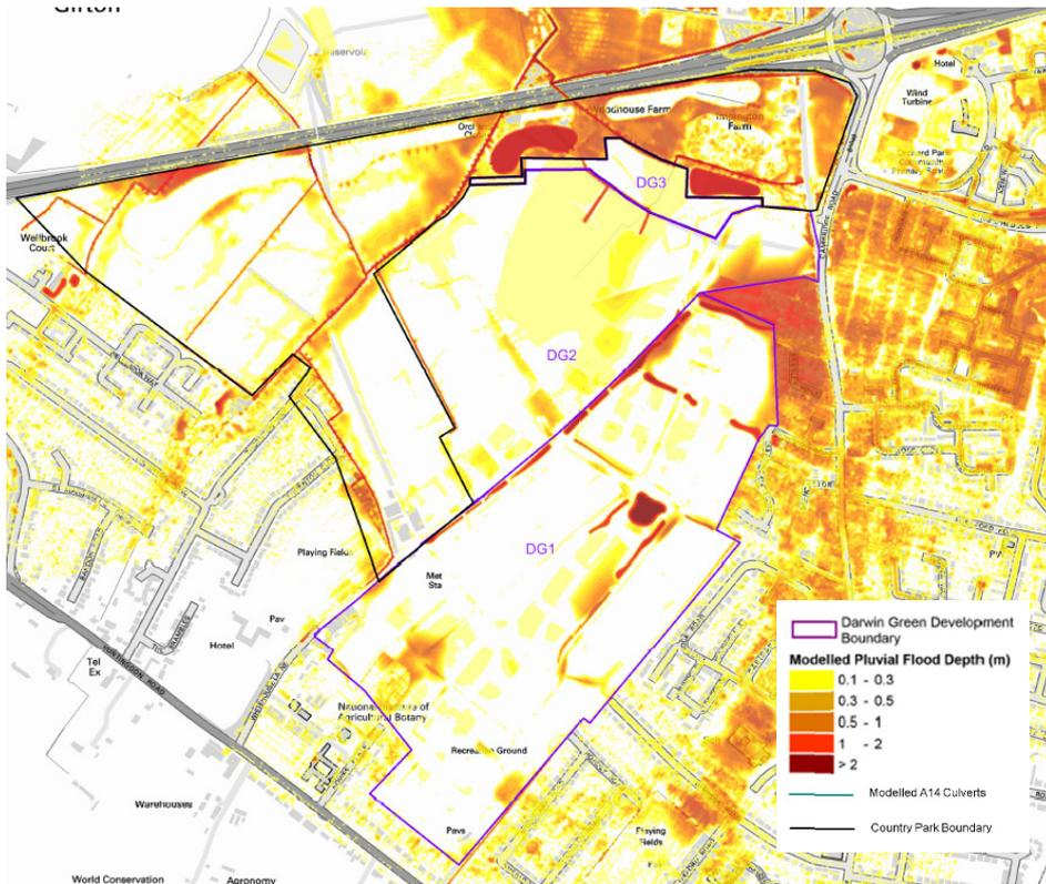
Figure 2 – Modelled Pluvial Flood Depths in the Post Development Scenario (for 1 in 100 year plus climate change event)
