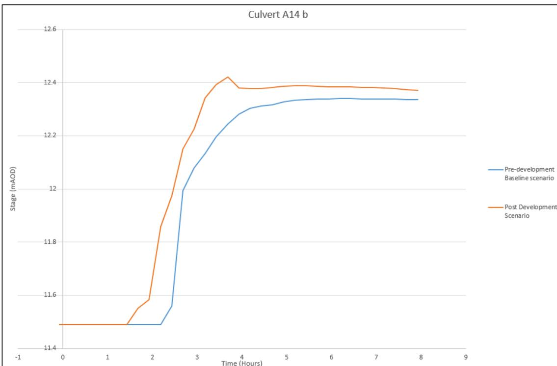
**Graph 4 – Water level at culvert A14\_b in both the Pre Development scenario and the Post Development scenario**
