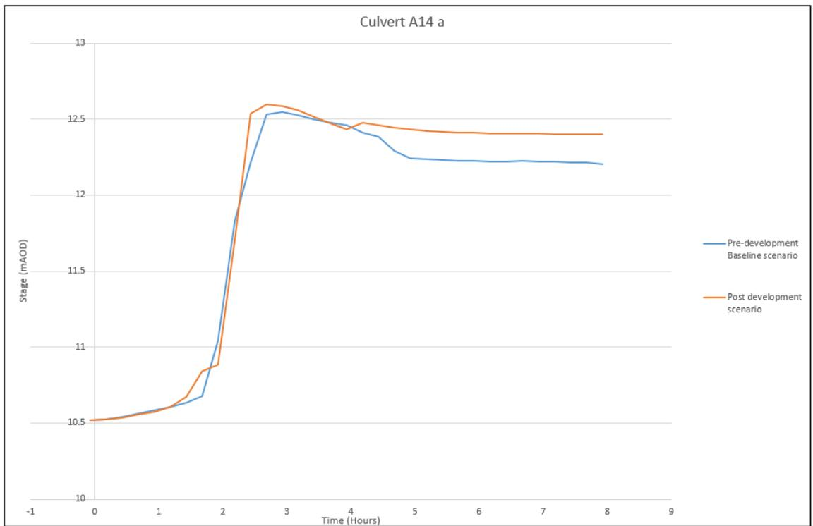
**Graph 2 – Water level at culvert A14\_a in both the Pre Development scenario and the Post Development scenario**
