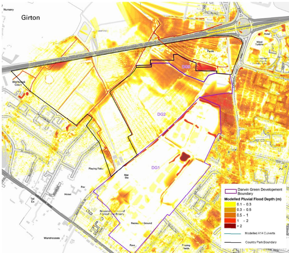
Figure 1 – Modelled Pluvial Flood Depths in the Pre-Development Scenario (for the 1 in 100 year plus climate change event)
