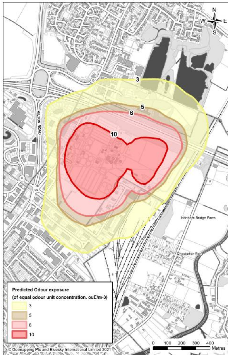
Figure 15.1: Odour exposure contours around CWRC - extracted from the Technical Note produced by CCC
