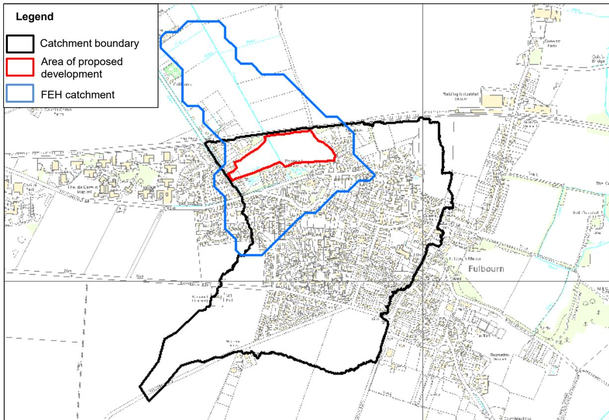
Figure 2.1: Catchment boundary from FEH and LiDAR
