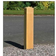
**BO1** Proposed Timber Bollard | Timber Bollard | Supplier: Broxap | Product Code: BX17 Painted - Square | Dimensions: 150x150mm x1000mm | Fixing: Fixed into concrete footing. Reflective bands in rebates. Granite setts surrounded.
