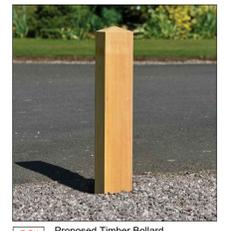
**BO1** Proposed Timber Bollard | Timber Bollard | Supplier: Broxap | Product Code: BX17 Painted - Square | Dimensions: 150x150mm x1000mm | Fixing: Fixed into concrete footing. Reflective bands in rebates. Granite setts surrounded.
